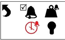
Alarms are on when the box next to the top left bell is checked.
