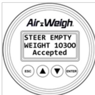
***Note that you must calibrate each axle group in order for the scale to be fully calibrated. Repeat the above steps for the Drive axle group.***
