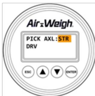
9. Using the up/down arrows <▲ ▼>, scroll to the proper empty weight identified from a certified scale ticket, then depress <ENTER>. The screen will briefly show Accepted to indicate its acceptance of the Empty Weight.
