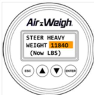
10. Press <ESC> to return to the PICK AXL menu and choose another axle for entering its Heavy Weight calibration. Make sure it flashes "ACCEPTED" at the bottom of the screen.
